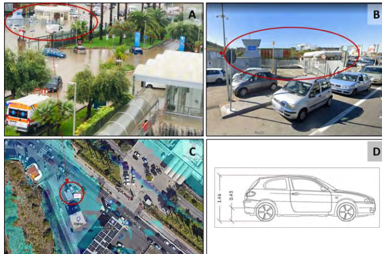
Figure 3 Example of how the HEC-RAS model testing phase is carried out. A) Observed runoff depths by using an image of the event occurred in October from Garibaldi-Nesima hospital security camera; B) Google Maps image; C) Simulated runoff depths by using HEC-RAS model; D) Fixed point, back bumper of an Alfa Romeo 147.
