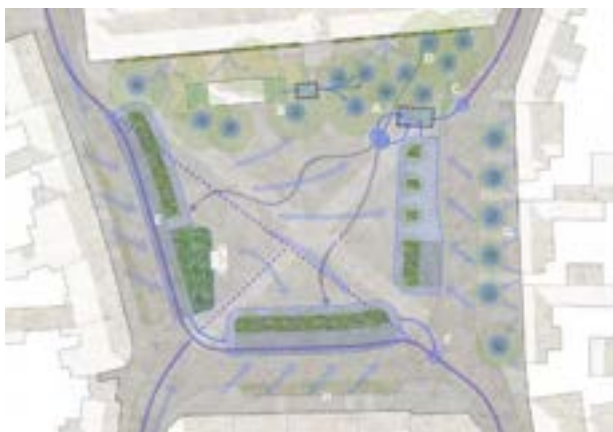
Picture 5 Movement of water through Zbraslavské square (atelier tečka architects, Grania s.r.o.)
