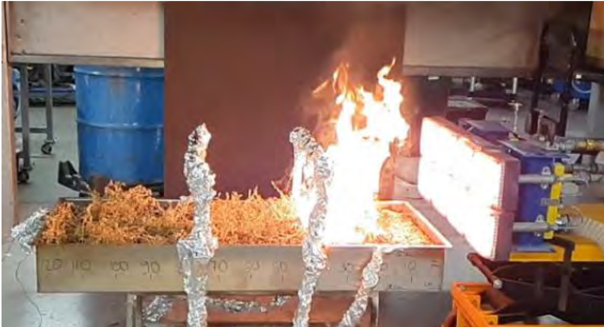
Figure 17 Trial to validate green roof flammability experimental setup and test sensor configurations
