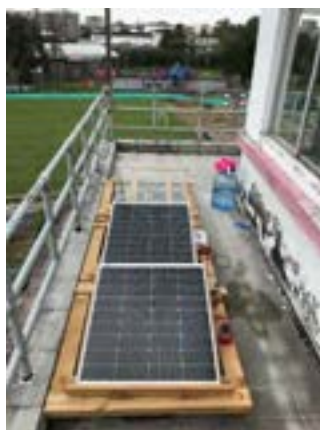
Figure 1. Experimental system with 2 solar panels, and a glass sheet supporting 90 small plates.
