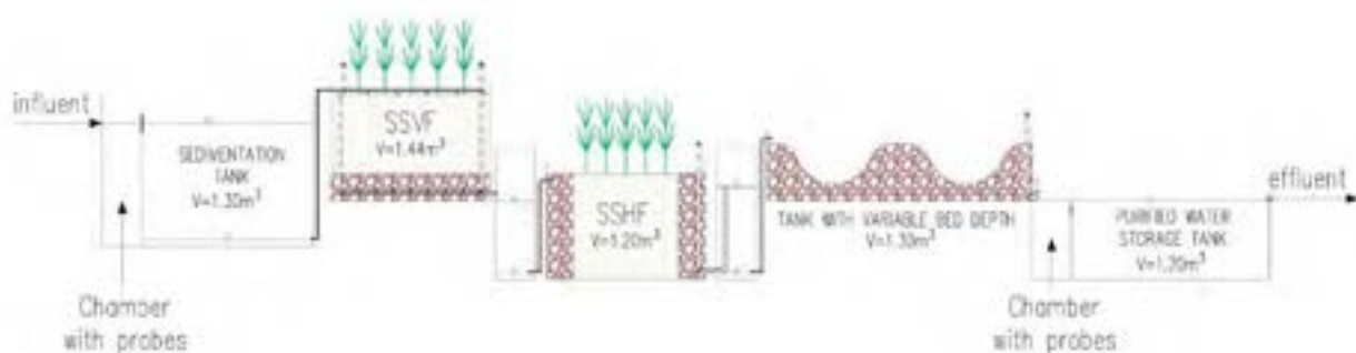
Fig. 1. Technological scheme of the MTWs. 1. Sedimentation tank, 2. 1st stage bed with the subsurface vertical flow (SSVF), 3. 2nd stage bed with the subsurface horizontal flow (SSHF), 4. reservoir with variable bed depth, 5. purified water storage tank; S1 and S2—water-collecting wells after SSVF and SSHF beds (Jakubowicz et al., 2022)
