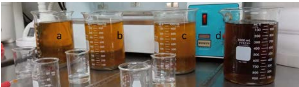
Figure 1. Reduction of colour in TV-A with Moringa oleifera seeds. a, b, and c, beakers with samples of coagulated tequila vinasse; d, initial tequila vinasse.
