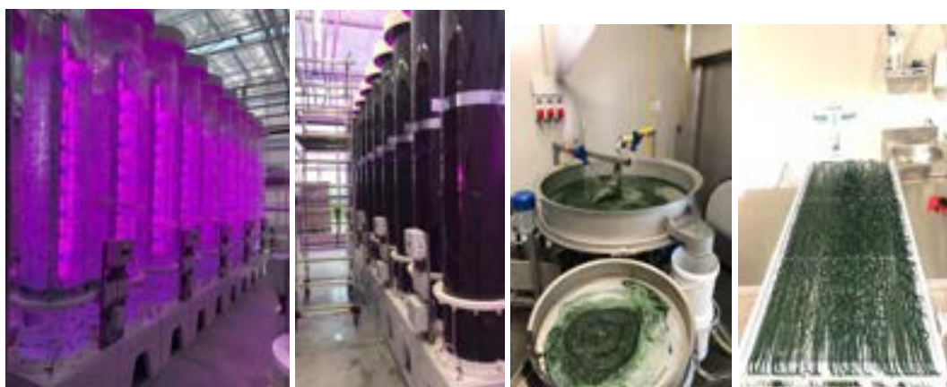
Figure 1: photobioreactor for growing of spirulina microalgae; spirulina microalgae preparation and drying
